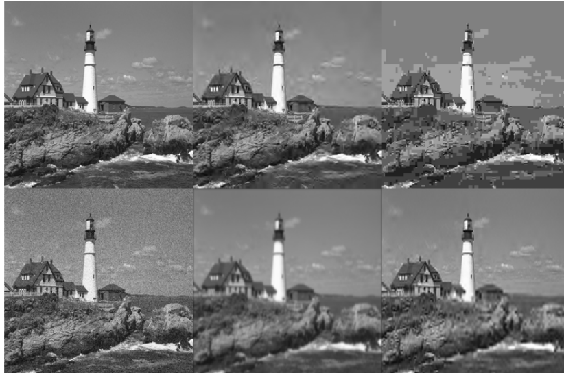
Figure 3: Reference image and five distorted images with different types of distortion in the LIVE dataset (JPEG2000, JPEG, WHITE NOISE, GBLUR, FAST FADING respectively).
