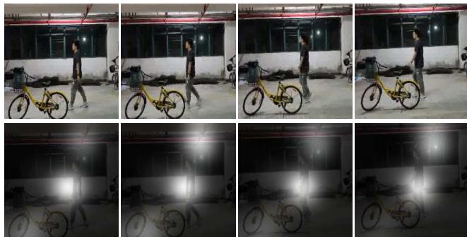
Fig. 7. Key frames of a video (upper row) and its attention mask (bottom row) generated by our method. The video contains a walking man and a stationary bike. It can be seen that the attention mask generated by our mechanism mainly focuses on the walking man instead of the stationary bike.
