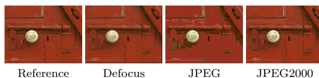
Fig. 1: Example of a reference image and three degraded images with blur or compression. The images are from the TID2008 dataset [24].
