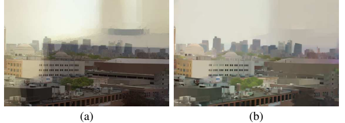
Fig. 1: Illustration of removing reflection with ghosting effect from a single image. (a) The image with reflection. (b) The result of removing reflection using the proposed method.
