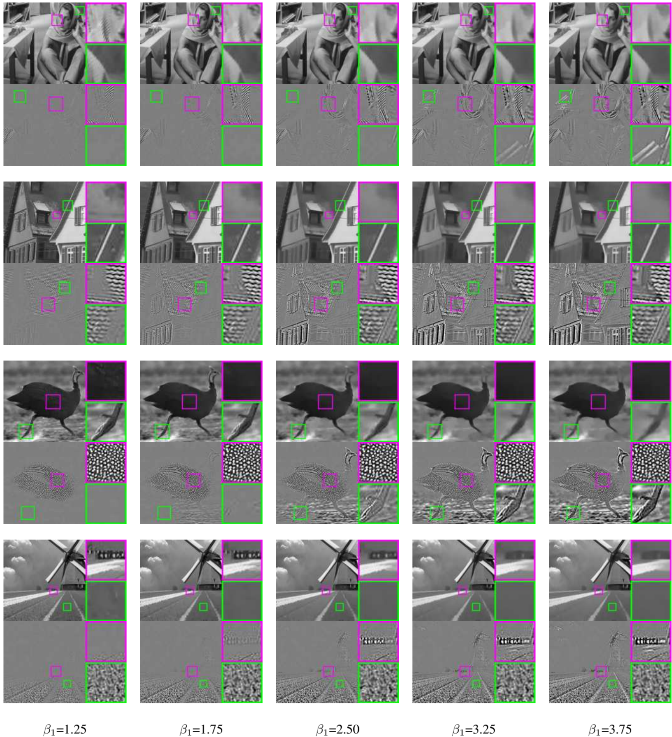
Fig. 23. Decomposition results of the proposed method on different images with \beta_1 varied from 1.25 to 3.75.
