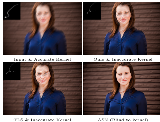
Fig. 13 Failure case of the proposed method when deblurring an image from Lai et al. ’s synthetic dataset in the presence of large kernel error.
