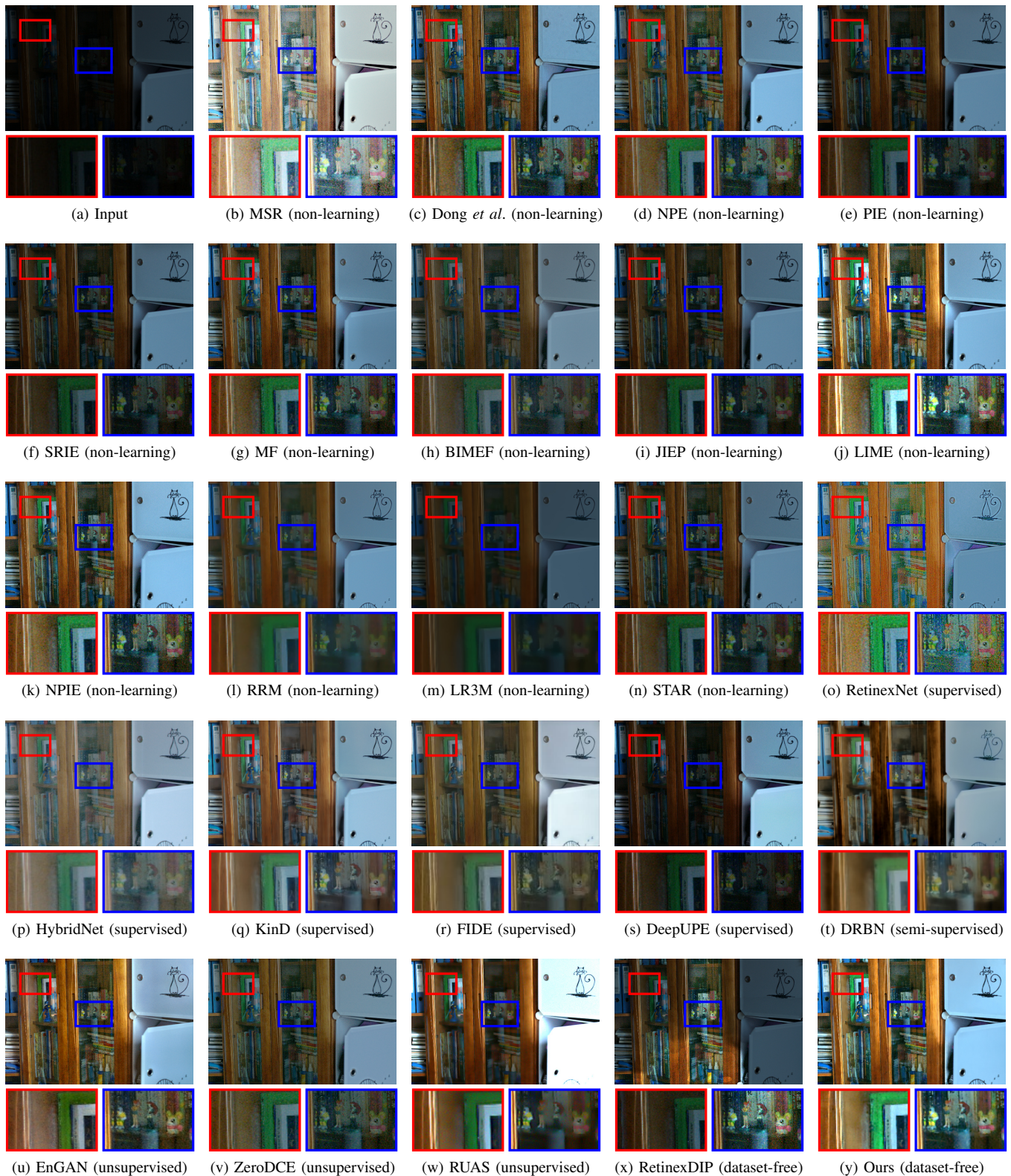
Fig. 13: Visual comparison of enhancement results on an extreme low-light image. LIME can restore vivid color. However, due to the lack of an effective denoising mechanism, the noise in the low-SNR regions is revealed in their results as shown in the red and blue boxes. In contrast, our proposed method is able to suppress noise in low-SNR regions while preserving color.
