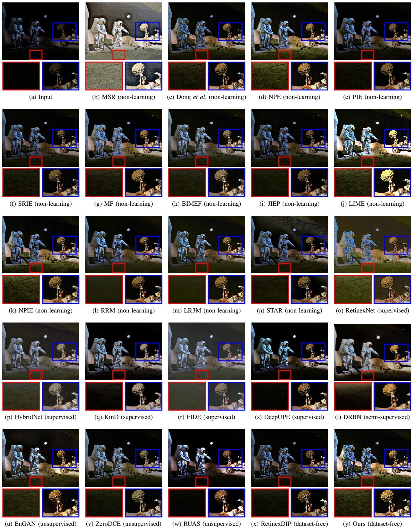
Fig. 14: Visual comparison of enhancement results on a low-light image, which shows that our proposed method can handle low-light images with negligible noise as well as the best methods. NPE, NPIE, EnGAN and our proposed method can well restore vivid color as well as fine details as shown in the red and blue boxes.
