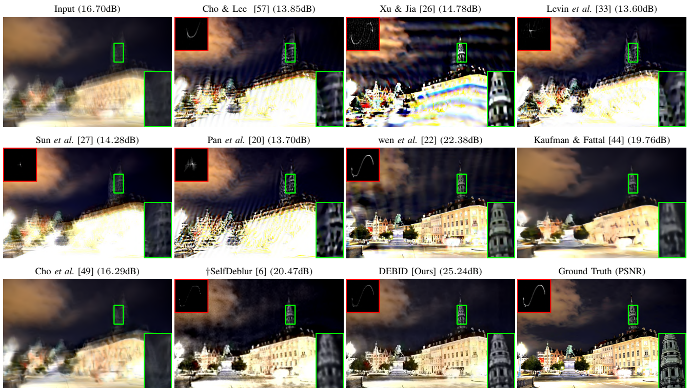
Fig. 6. Deblurring results of different methods on a saturated image from Lai et al. 's dataset. The estimated kernels are shown if available.
